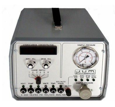
Fully complies with EN 12619, EN 13526 (TOC-EU), VDI 3481, 2. BlmSchV, 13. BlmSchV and 17. BlmSchV (TOC Germany), and EPA Methods 25A and 503 (USA)
