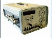
A rear panel toggle switch allows to chose between total organic carbon and methane carbon measurements. The disposable heated sample filter is easily accessible from the rear panel and no special tools required for a quick and easy sample filter change. All sample wetted components are integrated into the heated chamber.
